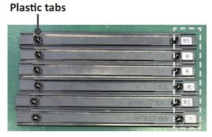
1. Place the Screen Bezel to the correct side of the screen to attach. Start from the left and move to the right.
