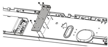
8. Further secure the Connector Plate with the two provided screws (M3 x 5 mm).
