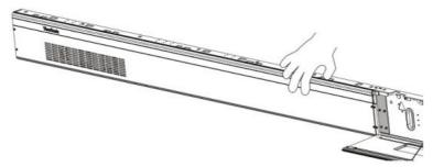
7. Secure the System Control Box panel with the Connector Plate using the provided screws (M3 x 6 mm).
