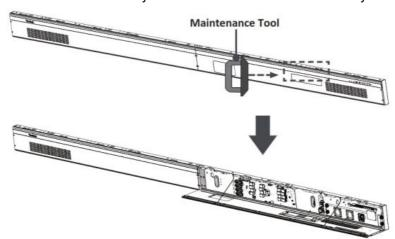
6. Remove the Left Cover by gripping the top edge of the Cover and pulling it toward you. The Left Cover should simply lift away.
