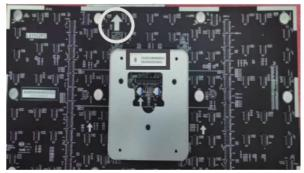
2. Attach the remaining LED Modules onto the Cabinets. Install from top left and move to bottom right, ensuring to match the corresponding numbers on the Module to the Cabinet. See Appendix C for further guidance on the LED Modules.
