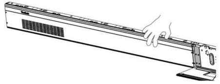
5. Secure the System Control Box panel with the Connector Plate using the provided screws (M3 x 6 mm).
