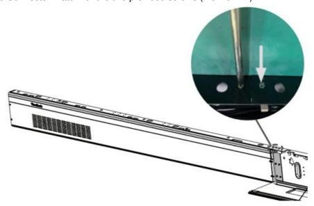
7. Install the short side of the Lower System Control Box Mount Bracket onto the top of the System Control Box with the provided screws (M3 x 6 mm).
