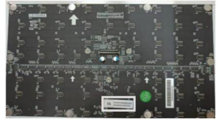
2. Attach the remaining LED Modules onto the Cabinets. Install from top left and move to bottom right, ensuring to match the corresponding numbers on the Module to the Cabinet. See Appendix C for further guidance on the LED Modules.
