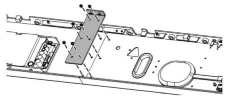
6. Further secure the Connector Plate with the two provided screws (M3 x 5 mm).
