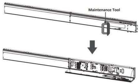
4. Remove the Left Cover by gripping the top edge of the Cover and pulling it toward you. The Left Cover should simply lift away.
