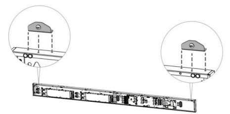
8. Install the provided screw (M8 x 16 mm) on the Lower System Control Box Mount Bracket. Thread the provided M8 nut onto the screw and fully tighten the nut.
