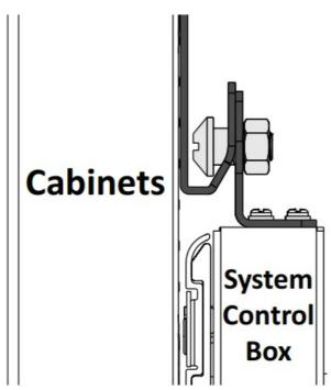
24. After installing the System Control Box, connect the Power and Network Cables from the System Control Box to each Cabinet. Start from the bottom and move to the top (see Appendix B for example system wiring diagrams, including wire colors and connection points).
