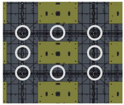
12. Assemble and install the remaining Cabinets in the same manner as the first two Cabinets. Ensure the Mounting Brackets sit securely on the Wall Mount Brackets, and that the Cabinets are properly secured together.
