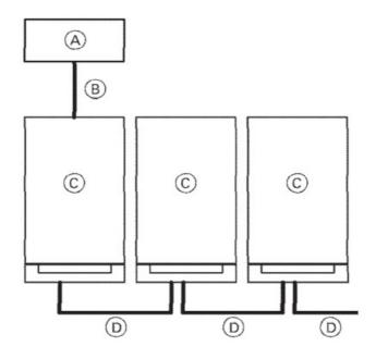
Note: The total length of BUS cables B and D should not exceed 164 ft. (50 m).
