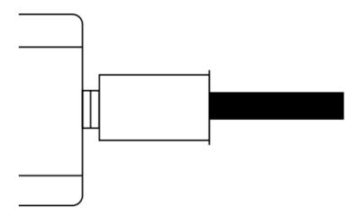
• **b.** Insert the socket remover as far as possible into the security socket. Turn counter-clockwise.
