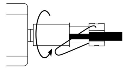
• c. Remove the security socket and coaxial cable from the device. If there is a filter in the socket, remove it using the socket remover.
