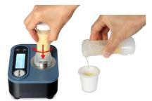
4. Add 200 μL ONE Diluent into a new strip test vial, add 100 μL of filtered extract into the same vial, cover and mix well by shaking 3 times.
