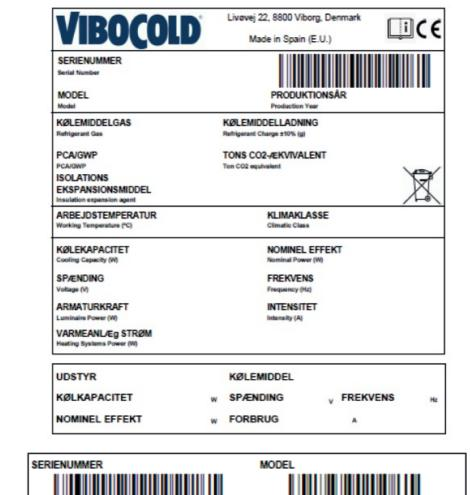
Apart from the identifying data of the unit, information relating to the gas refrigerant and electrical voltage to which the unit must be connected is also displayed.
