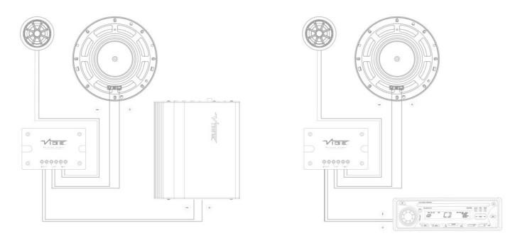
• Connect the speaker to the speaker wiring in the vehicle ensuring that correct polarity is observed.
