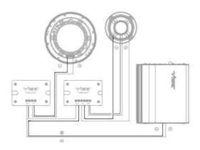
• Connect the speaker to the speaker wiring in the vehicle ensuring that correct polarity is observed.
