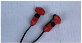
19. Connect the T-Crimp connectors to the stereo front speaker output wires. Take special care to ensure the polarity is correct so power correctly flows through the tweeter crossover. If unsure refer to your stereo user guide or wiring diagram. (Tweeter wiring, Black/White – Positive +, Black – Negative **Note:** Failure to complete this step correctly may result in damage to the tweeter
