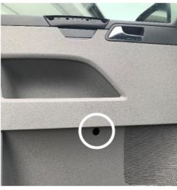
5. Remove the three T25 Torx screws located along the bottom edge of the door card. Once removed, use a trim
