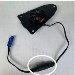
22. Reconnect the tweeter in the vehicle and secure the tweeter mount using the T15 screw previously removed.
