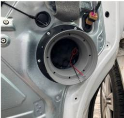
14. Connect the speaker spade terminals to the woofer ensuring the polarity is correct (Red Positive +, Black Negative -) Line up the holes and silicone baffle and use the screws provided to secure to the speaker adaptor
