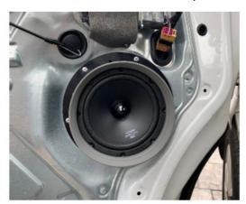
Test the speaker and re-install the door card. Re-installation is a reversal of the removal process.
