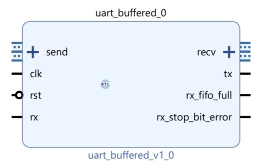
All three modules have built-in flow control through the use of ready/valid handshake signals. And because the signal naming scheme matches the Xilinx AXI standard, the send and recv ports will appear as bus interfaces in the Vivado Block Design editor, as shown in the image above.
