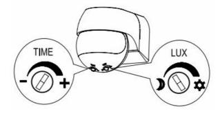
**Note:** when testing in daylight, please turn LUX knob to (SUN) position, otherwise the sensor lamp could not work! If the lamp is more than 60W, the distance between lamp and sensor should be 60cm at least.
