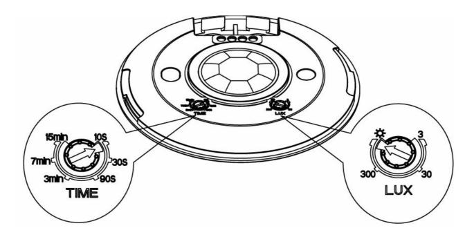
**Note:** when testing in daylight, please turn LUX knob to (SUN) position, otherwise the sensor lamp could not work! If the lamp is more than 60W, the distance between lamp and sensor should be 60cm at least.
