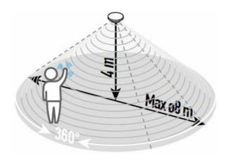
Height of installation: 2.2-4m Detection Distance: Max.8m
