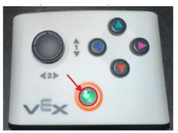
7. LED should turn orange once the One Stick Controller has entered pairing mode.
