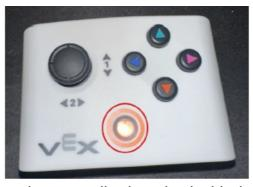
8. LED should blink green once the controller is paired with the AIM RoboThe t.
