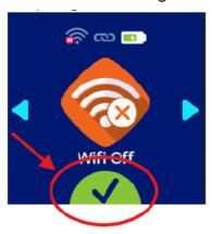
6. Verify the Robot is in Bluetooth mode by checking the signal strength icon.
