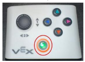
9. AIM Robot should show signal strength in the top left corner when connected to the Once Stick Controller.
