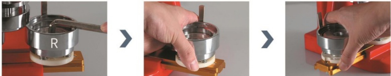
Figure 2: loosen the screw of the mold slightly with a hexagon wrench, rotate the whole die to an angle, and then conduct a pressure test until the upper and lower dies are aligned, and then tighten the screws.
