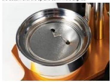
5. Hand holds the machine body, right hand down press the handle until up and down mold merged to bottom, now the upper mold hinge is in merged state, and the pin passes through the hole.
