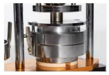
4. Put the plastic back plate into the eft mold (Attention: The pin should be level without protruding. The upside words upward placed according to the mold side triangle indication mark), rotate the down mold clockwise to the bottom until the up and down mold aligned.
