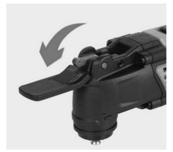
2. Extract the necessary functional accessories, align the positioning holes on the accessory's installation end with those on the installation bracket, and firmly secure the components in **place**.
