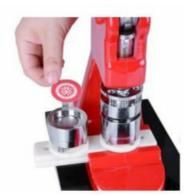
1. Place metal badge top (rim down) in left hand die in the circular slot. Cover with cut out print (printed side up) and one plastic film.
