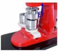
2. Align die set into the body groove. The top die may need to be lifted before sliding die set.
