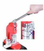
3. Place pinned back (zigzag side of pin showing) in right hand die. Press down the handle to complete assembly. There must be no gap in the top die when you press down the handle.
