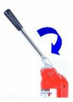
3. Secure die set with two small nails. Screw the handle to the body.
