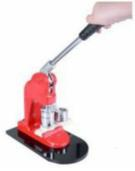
2. Press down the handle to complete assembly. Be sure there will be some gap in the top die when you press down the handle.
