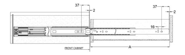
**STEP1:Cabinet Installation For Ball Bearing**
