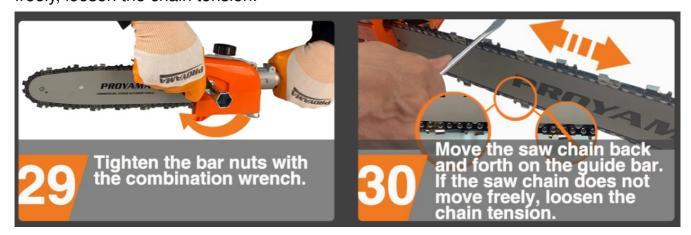
NOTE1: The chain is tensioned correctly the weight of the chain does not cause it to sag below the guide bar (with the chain saw sitting in an upright position), but the chain still moves freely around the guide bar(FIG 12).
