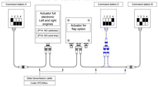
This installation scheme is valid for systems with up to 3 command stations and 2 engines and gearboxes, full electronic
