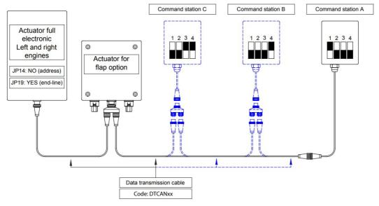
This installation scheme is valid for systems with up to 3 command stations and 2 engines and gearboxes, full
