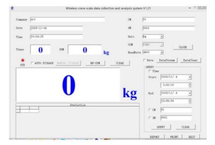
Now the computer can receive the data from the 180 indicator. After the test is stable, the STB light will become
