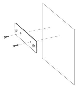
5. Attach the HWC-1 onto the bracket as shown below.
