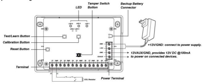
The Power Terminal (Z1~Z9 zones) inputs allow existing wired sensors to be connected to the HWC-1 Converter:
