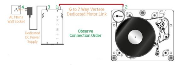
Attach the record player end 7-way connector to your record player motor input socket Only applicable to 2021 models onward – record players with 7-way motor power input sockets. Please refer to your record player user manual.
