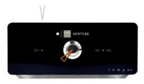
• Press and hold the button for 1.5 secs to stop and the Speed indicator LED will turn off.
