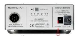
Plug in the dedicated DC power supply and back panel Red LED will illuminate to indicate DC power connection.
