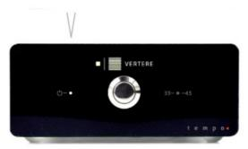
• Front panel power indicator LED will also illuminate White. (Tempo is factory set to Mode 1)
