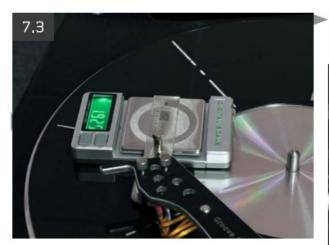
Adjust the Vertical Tracking Angle (VTA) so that the cartridge body is parallel to the record surface.
