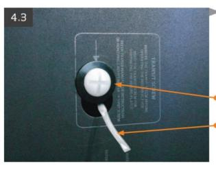
Remove the chassis from the carton and rest it on its left side to gain access to the underside. Unscrew and remove the underside transit screw. If necessary, use a coin to assist loosening the transit screw.
