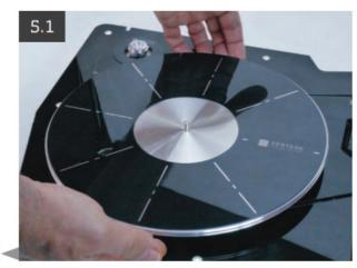
Lower the platter gently on to the bearing spindle. Keep the platter horizontal as it is lowered.
