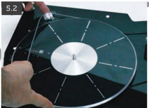
Check that the drive belt is located correctly in the pully and platter grooves.
