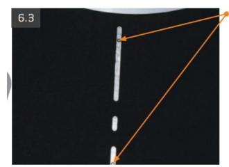
When the stylus is positioned on each alignment point, the end of the head-shell and the cartridge should align with the radial platter line. Move the cartridge to adjust. ■
