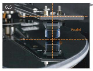
Check the cartridge azimuth.
