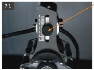
Fine adjust the tracking force by moving the balance weight: backwards to reduce tracking force, forwards to increase.
