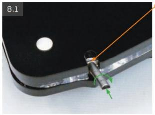
Ensure that the hinge mounting bars are oriented with their flat sections facing downwards. Raise the hinge mounting bars to the vertical position.
