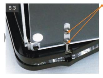
Position the lid in place and initially secure it with one dome-head Allen screw on each side. Do not fully tighten the screws. Insert the second screw each side then fully tighten all four to secure the lid. Do not over-tighten the screws.
