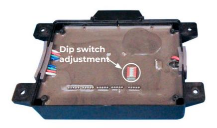
The control module has the ability to turn off zones if an input line to the controller is activated. If the disable line is held at the input voltage (5-24 volts), Zones one and two will be turned off. This feature can be used if you want to deactivate the zone lights on the outside of the boat when in motion. By default, only zones one and two are turned off.
