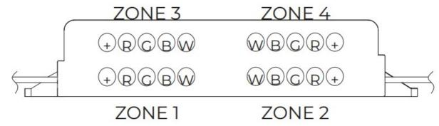
4. WIRING DIAGRAM: Follow the wiring diagram below to wire the module to your system. Note: Maximum replacement fuse size is 25 amps.
