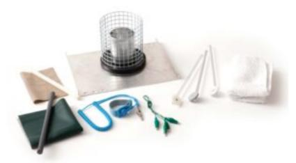
Use the sensor with a Faraday pail to investigate charging by induction. Bring a charged object near the pail. What charge is measured? Ground the pail and remove the charged object. What charge is measured?
