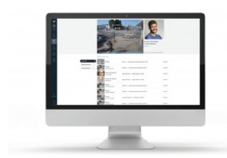
Command, Verkada's cloud-based management platform, is designed to deliver simple access and management for all cameras and users across every site from virtually anywhere in the world. From Command, users can set up new cameras, create new sites, manage settings, access live and archived footage, manage users, and access the advanced features powered by Verkada's edge-based analytics.
