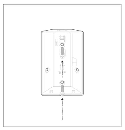
• Mount the bracket on a flat surface or in a corner with the supplied screws and wall anchors.
