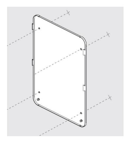
Place the sheet metal enclosure over and onto the mounting plate tabs.
