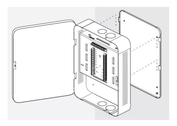
Fasten the two security torx screws to secure the enclosure to the mounting plate.
