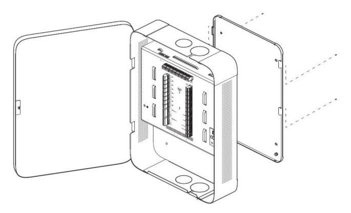
Drill four 5/16" Ø holes into the wall. Insert the drywall anchors into the holes. Fasten the mounting plate onto the wall by installing the mounting screws into the wall anchors.
