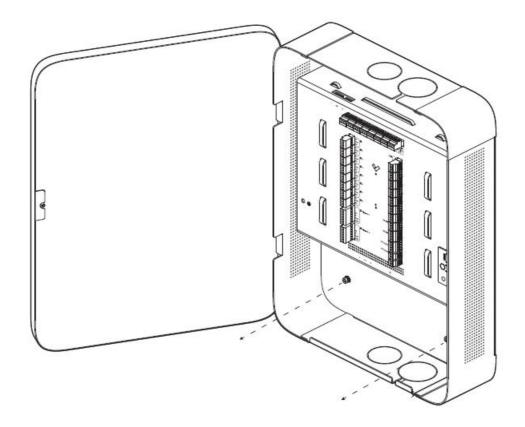
Once the security screws are fully removed, slide the mounting plate down and away from the main enclosure.
