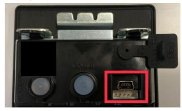
12. Plug in to the "Program" port on the back of the lock underneath the battery cover using a USB to mini USB cable.
