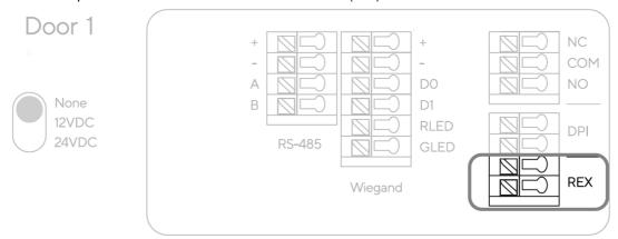
The REX can be configured to release the lock in Verkada command; most commonly seen in electromagnetic locks. The REX unlock time can also be configured.
