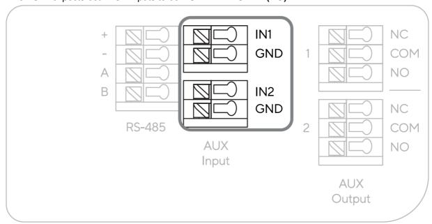
With the AC41's AUX inputs you can hook up devices such as intercoms and buttons into the auxiliary cassette of the AC41, and all associated unlock events will be logged in Command.
