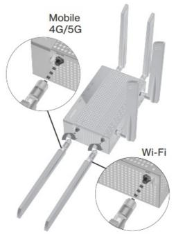
3. **Position antennas:** For the best reception, position the antennas so that they are in an upright position as illustrated. Once completed, please plug in and power on the device.
