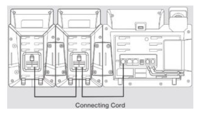
**Note:** You can connect six modules at most. You just need to connect the Ext in jack of the previous module and the Ext out jack of the next module using a connecting cord.
