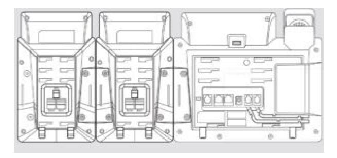
**Note:** The T46G IP phone can support six expansion modules at most. But if you use more than two expansion modules, you need to connect an additional power adapter to any one of the expansion modules.
