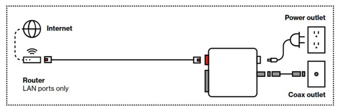
Use the MoCA Ethernet Adapter as a connector between the coax outlet and your personal devices.
