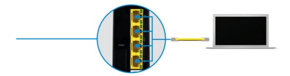
Connect the Ethernet cable to any YELLOW LAN port on the router, then to the Ethernet port on your computer.
