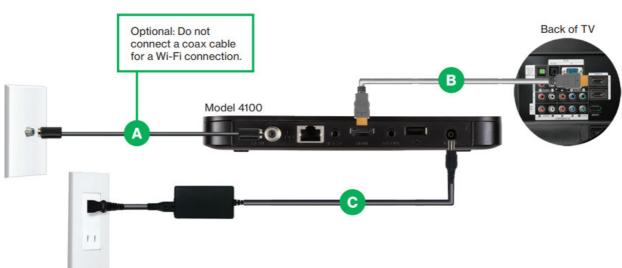
A. Connect to Fios TV via a Wired or a Wi-Fi connection
