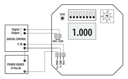
Wait five seconds, then press and hold the ZERO pushbutton for two seconds or provide contact closure on the AUX ZERO terminal. This will reset the output and display to zero pressure. For best accuracy, press the ZERO button while both ports are open to atmospheric pressure. To protect the unit from accidental zero, this feature is enabled only when the detected pressure is within about 0.5 in. WC (125 Pa) of factory calibration. Connect desired external tubing to the PX3.
