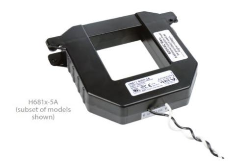
H681x-5A split-core current transformers (CTs) provide secondary amperage proportional to the primary (sensed) current. For use with power meters, data loggers, chart recorders, and other instruments, the H681x Series 5 Amp CTs provide a cost-effective means to transform electrical service amperages to a 0 to 5 Amp level compatible with monitoring equipment.
