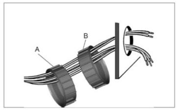
3. For 85 mm instruments, the fastening nut can be mounted at position A or B. This allows you to fix the gauge in different panel bores.
