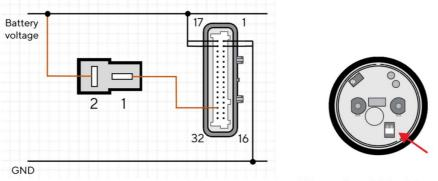
Make sure the switch heads towards the outside of the sensor.
