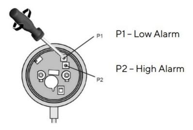
If the Low alarm is not needed, carefully turn P1 clockwise to the limit. If the High alarm is not needed, carefully turn P2 counterclockwise to the limit.
