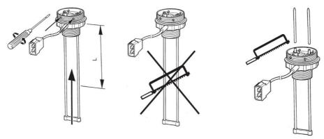
Loosen the screws in order to adjust the length of the rods.
