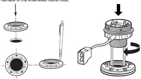
Use the flange to mark the placement of the drill holes. Place the soft rubber seal between the flange and the tank. When the flange is mounted on the tank, screw in the sensor from the top.
