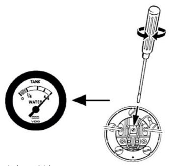
To calibrate the sensor, fill the tank completely.
