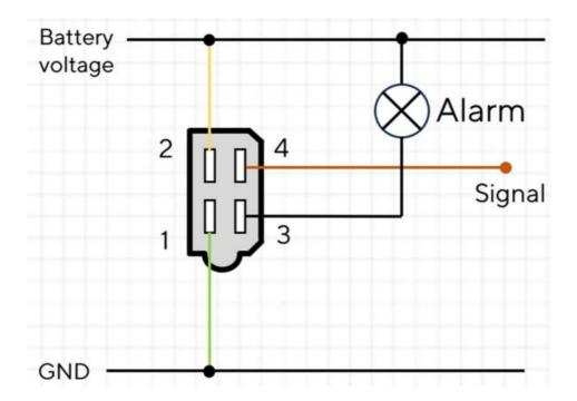
The -90X-Sensors provide an alarm output.
