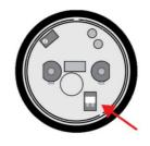
Make sure the switch heads towards the center of the sensor. veratron AG
