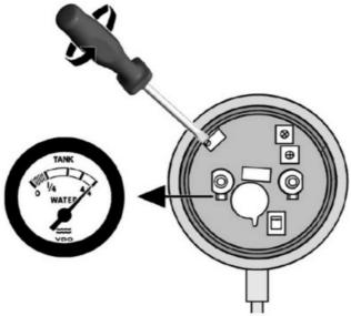
Make sure the switch is in the correct position depending on the instrument, that reads the signal. (See the according drawings in the chapter Electrical Installation > N02-24090X .)
