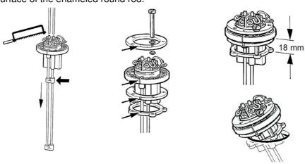
After shortening the rods, readjust the clamp to the middle of the new height.
