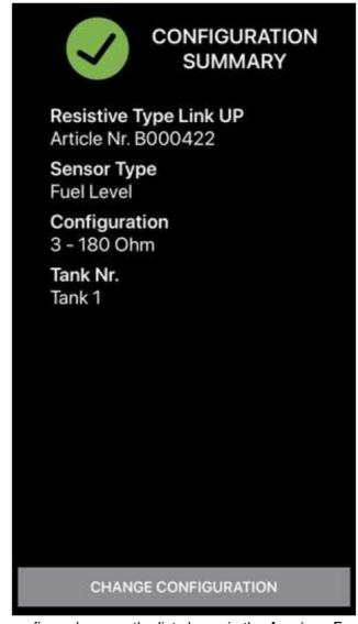
3. Select the sensor type to be configured among the list shown in the App (e.g. Fuel Level). Then choose the calibration for the selected sensor (e.g. 3-180  $\Omega$ ) and its instance (e.g. Tank 2) so that the Link Up gateway will correctly transmit the value over NMEA 2000 $^{\circ}$ 8.
