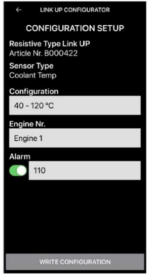
4. To upload the configuration, simply "tap" the smartphone again onto the Linkups wireless area, as described in step 1.
