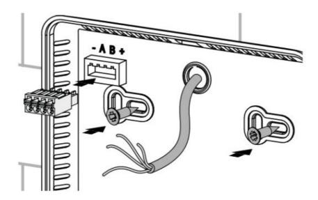
4. Connect the power supply cable wires according to the diagram of the electrical connections.
