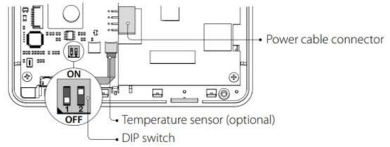
The temperature sensor is an optional device that measures the temperature in the room. If physically present in the panel configuration, select the "Sensors in control panel" item in the control panel menu.
