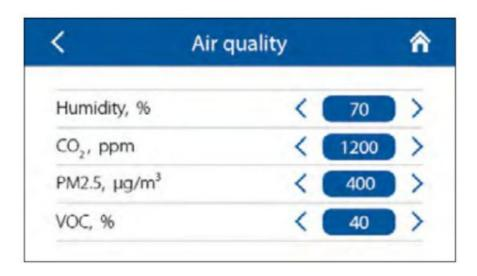
Set threshold values for the humidity, CO2, PM2.5, and VOC sensors.
