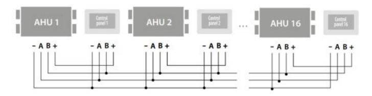
ATTENTION! CONNECTING MORE THAN 3 CONTROL PANELS TO A SINGLE AHU REQUIRES AN EXTERNAL POWER SUPPLY UNIT.
