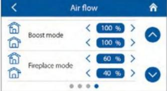
This menu enables setting the airflow rate for pre-set speeds 1, 2, 3.. as well as the Standby, Boost, and Fireplace modes.
