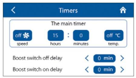
Once the Main timer is enabled via the Main page menu, the air handling unit temporarily switches to the following settings:
