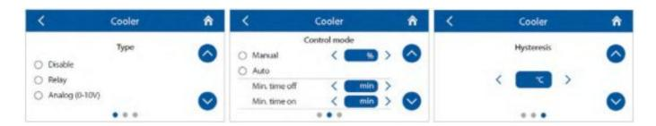
Select the cooler type (discrete/analog) and its operation mode.
