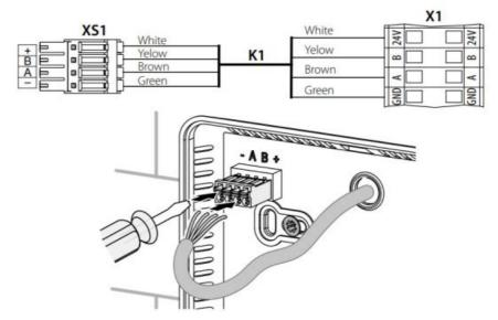
5. Remove the connector with the cable from the bracket and connect it to the female connector on the circuit board.
