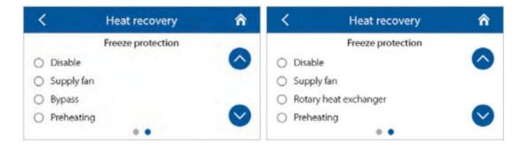
Depending on the particular AHU configuration use this window to select the necessary control mode for the bypass/rotary heat exchanger with discrete or analog control.
