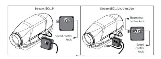
The fan speed without options can be controlled by voltage, as well as by thyristor controllers.
