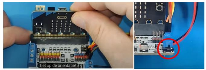
• Press the RESET button on the back of the Micro Bit, and the OLED screen should light up. Now follow the instructions on the screen.
