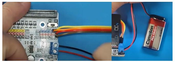
• Connect the Micro Bit and set the ON/OFF switch of the motor board to ON.
