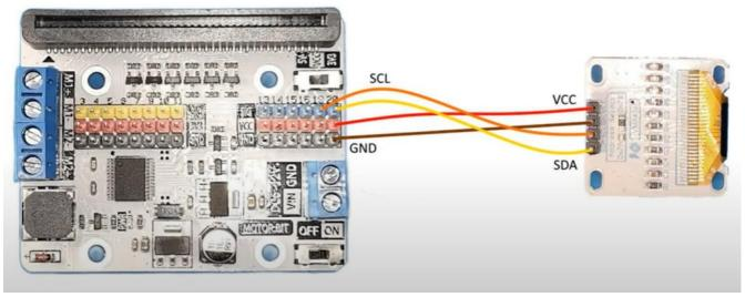
• Make sure the Slide switch is set to 3V3
