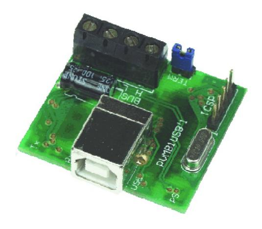
• Allows interfacing of the VELBUS system to a PC
