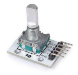
The VMA435 is a digital rotary encoder module that provides an indication of how much the knob has been rotated and in what direction. It is designed for stepper and servo motor control. The module has a working voltage of 0-5 V and is an incremental encoder type. It is made of PCB and brass, with a cycles per revolution (CPR) of 20. The dimensions of the module are 26 x 19 mm and it weighs 10 g.
