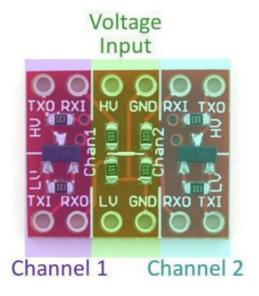
The middle section of the board serves the high and low voltages. Supplying voltage to all four of these pins is required.
