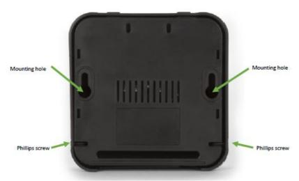
The receiver can easily be mounted against a wall or ceiling with the 2 mounting holes in the back of the case. The mounting holes have a diameter of 6,3 mm and the centre points are 62,9 mm apart from each other. Loosen the 2 Phillips screws on the two sides of the case to open the enclosure.
