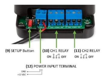
If the power supply is successfully connected, the power LED (5) will light up and the TUYA LED (6) will start flashing after a few seconds. Please do not connect the CH1 RELAY and CH2 RELAY terminals (10 & 11) or close the enclosure yet. We first need to pair a transmitter or connect to the TUYA IoT cloud.
