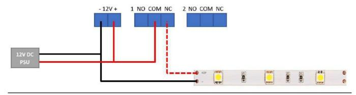
Example 2: device with a different power supply voltage as the VM130V2SET with NO contacts
