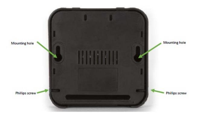
The receiver can easily be mounted against a wall or ceiling with the 2 mounting holes in the back of the case. The mounting holes have a diameter of 6,3 mm and the center points are 62,9 mm apart from each other. Loosen the 2 Phillips screws on the two sides of the case to open the enclosure.
