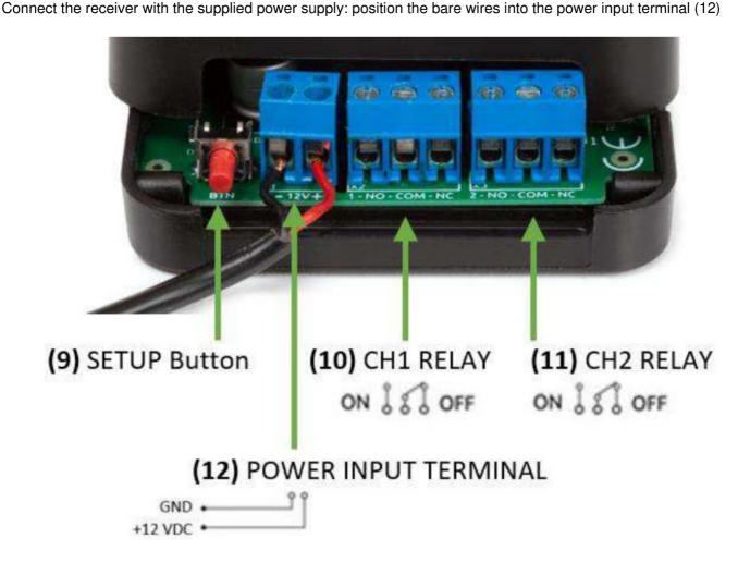
If the power supply is successfully connected, the power LED (5) will light up and the TUYA LED (6) will start flashing after a few seconds.
