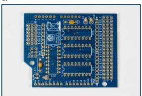
• RN1, RN2, RN3: resistor array 100k
